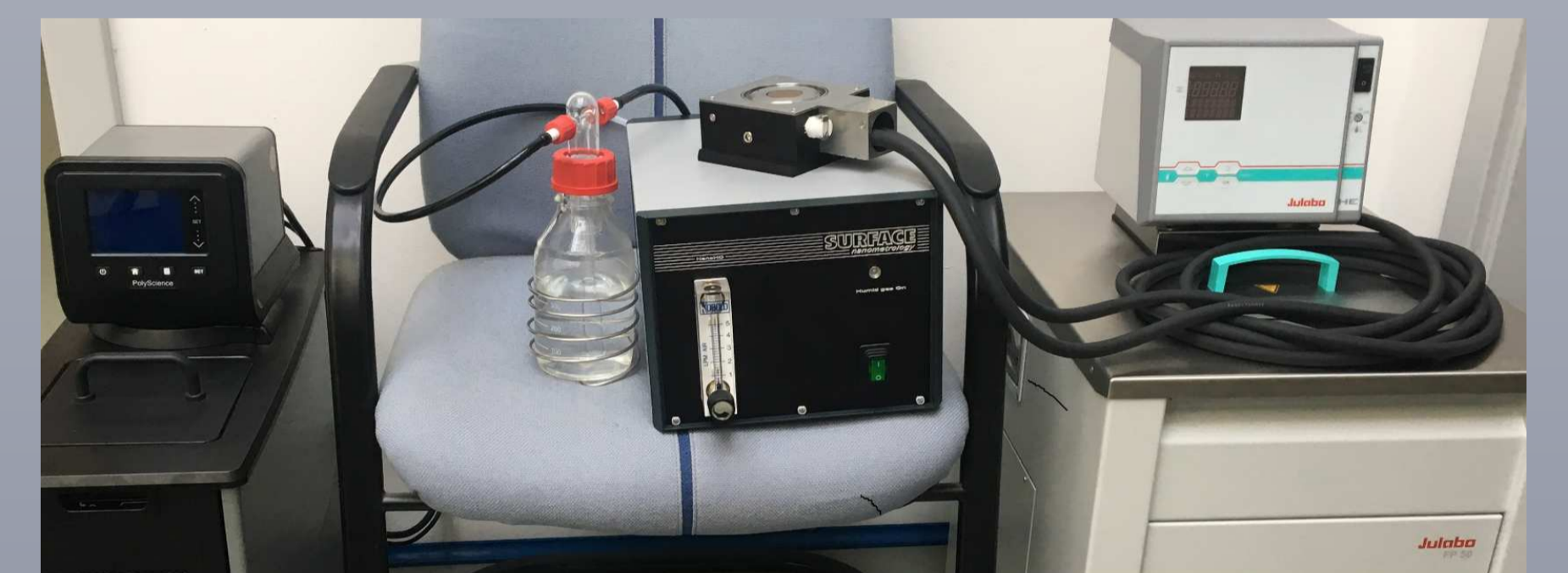
Left: Circulating chiller to stabilize nanoindenter temperature Center: Humidity controller with heating cooling humidity stage Right: Circulating chiller for large sample temperature range
