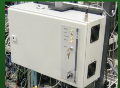
Laser with power supply in its control box close to the vacuum chamber
